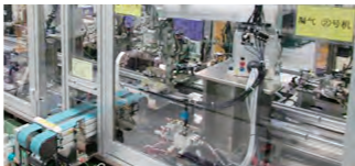
Automated motor performance inspection machine
