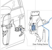
Image of a motor mounted to a door closer and the benefits of motorization
